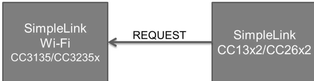
**Figure 9. Block Diagram of One-Wire REQUEST Coexistence**
