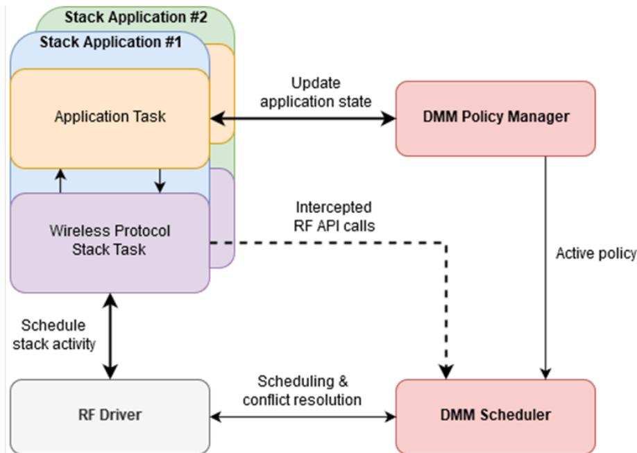
**Figure 11. DMM Architectural Overview Block Diagram**
