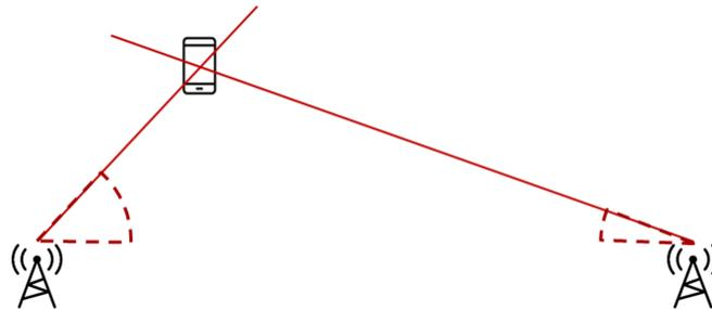
**Figure 6. Triangulation Using Connected AoA**
