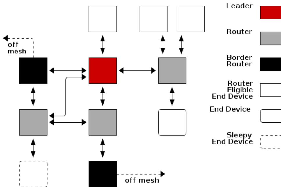
Figure 4. A Typical Thread Network
