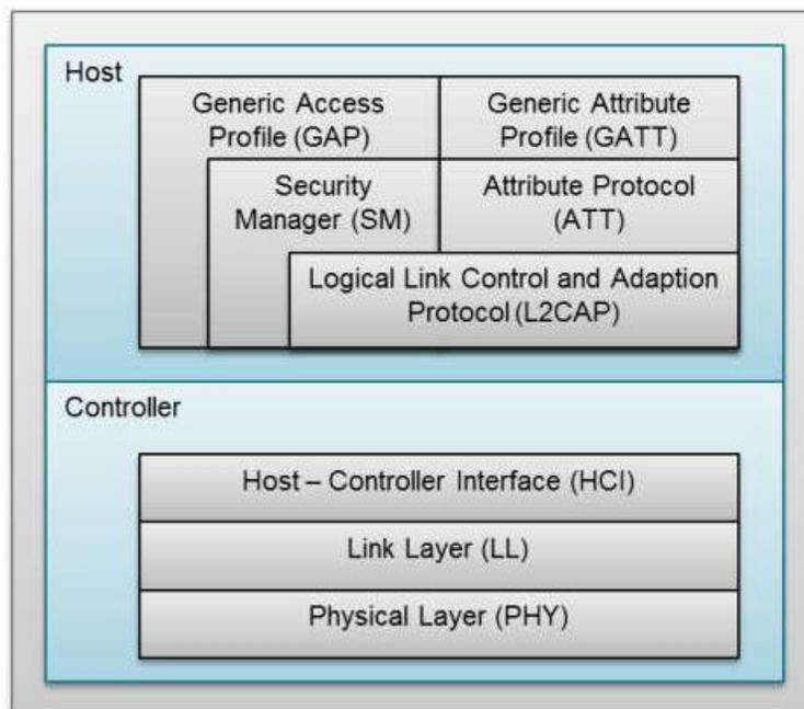
**Figure 5. Bluetooth Low Energy Protocol Stack**
