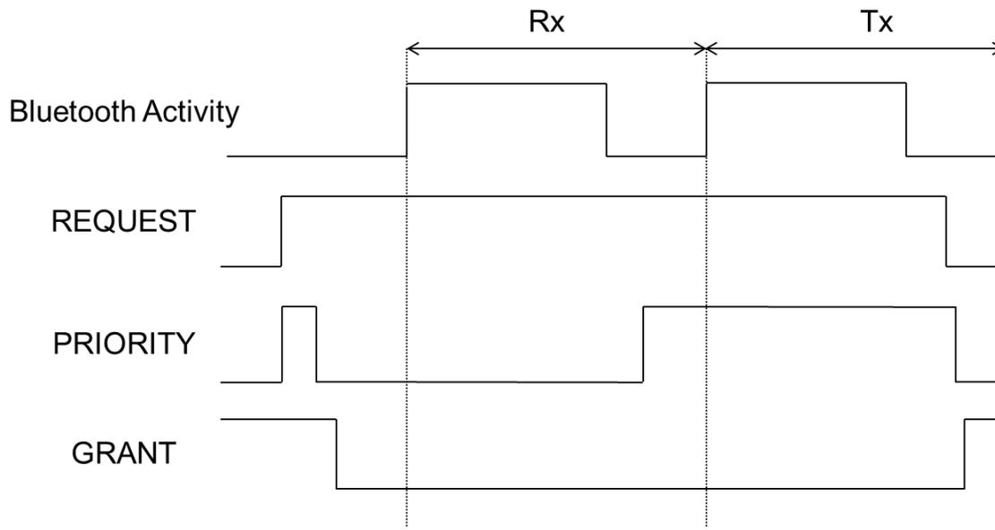
Figure 8. Timing Diagram of the Three-Wire Coexistence Signals
