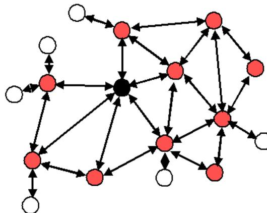
**Figure 3. A Typical Zigbee Network**
