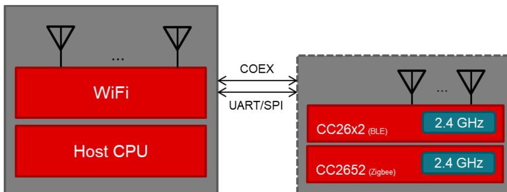
Figure 1. WLAN Solution Using a Two-Chip CC26x2 Solution
