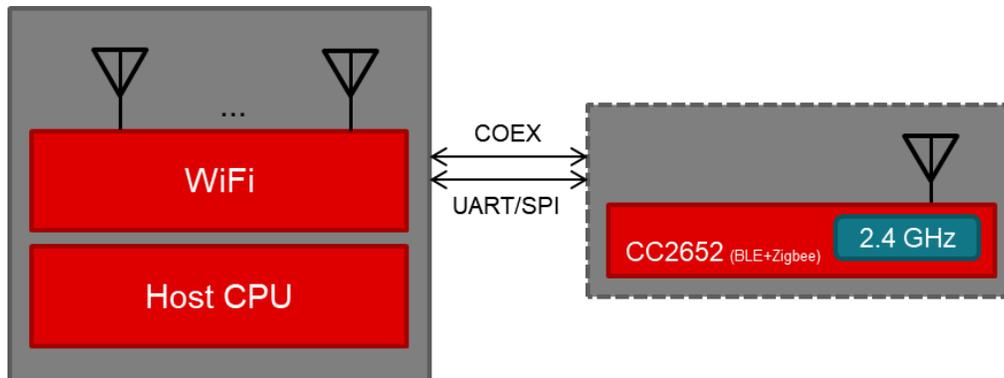
**Figure 2. WLAN Solution Using a One-Chip CC2652 Solution**
