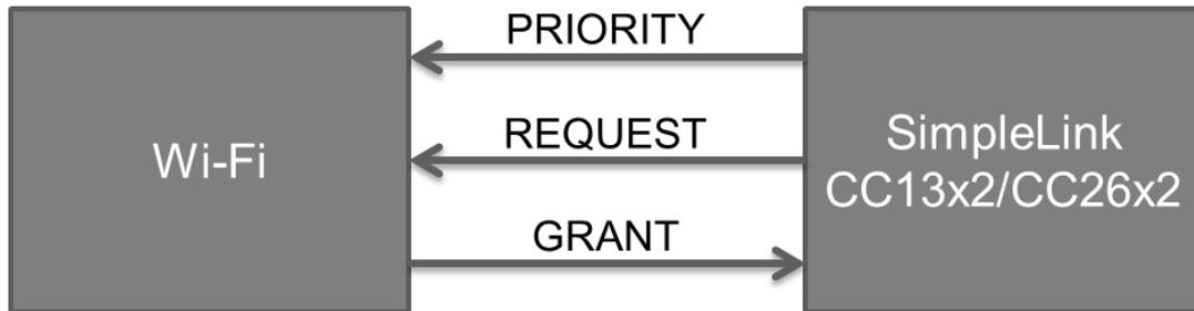
Figure 7. Block Diagram of Three-Wire Coexistence
