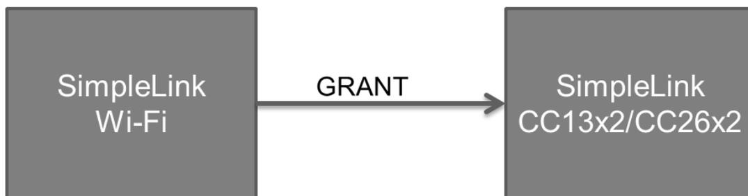
**Figure 10. Block Diagram of One-Wire GRANT Coexistence**
