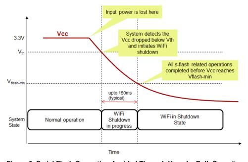
Figure 6. Serial Flash Corruption Avoided Through Use of a Bulk Capacitor
