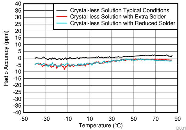
Figure 2. Crystal-Less Device With Varying Solder Amounts
