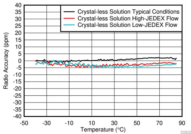
Figure 3. Crystal-Less Device With Solder Profile Changes
