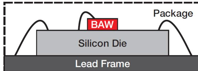
**Figure 1. CC2652RB Package Fabrication**
