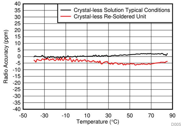
Figure 6. Re-Soldered Crystal-Less Device
