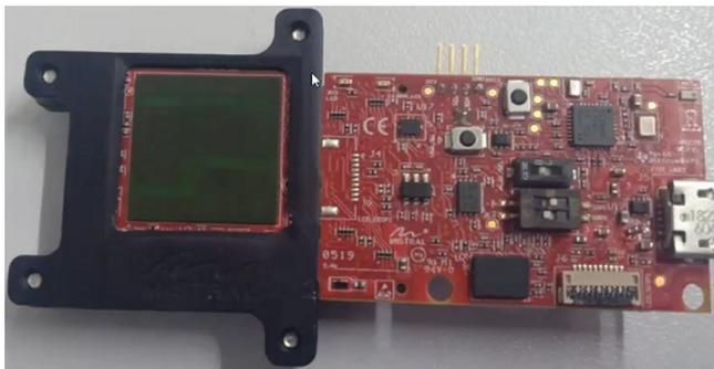
Figure 14. Top Side of the EVM With Heatsink Mounted
