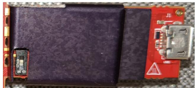
Figure 10. Bottom Side of the EVM With Heatsink Mounted
