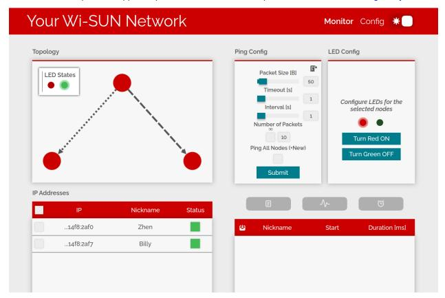
Figure 5. FAN Visualization in wfantund Webapp
