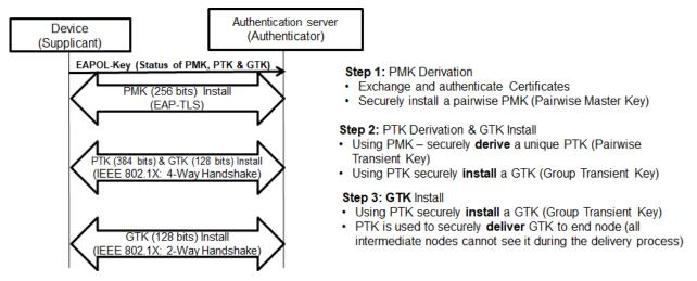
Figure 3. Security Key Exchange Mechanism in Wi-SUN®
