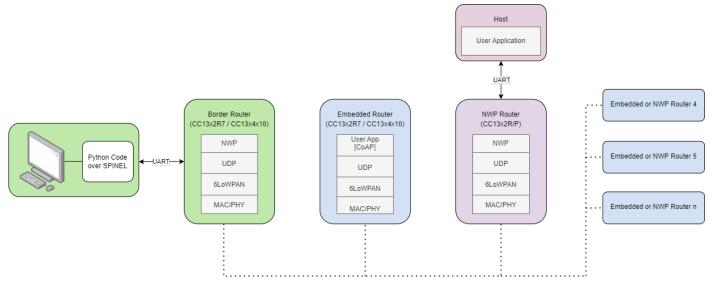
Figure 1. Available Network Architectures With Border Router and Routers Using NWP Implementation and Embedded Routers
