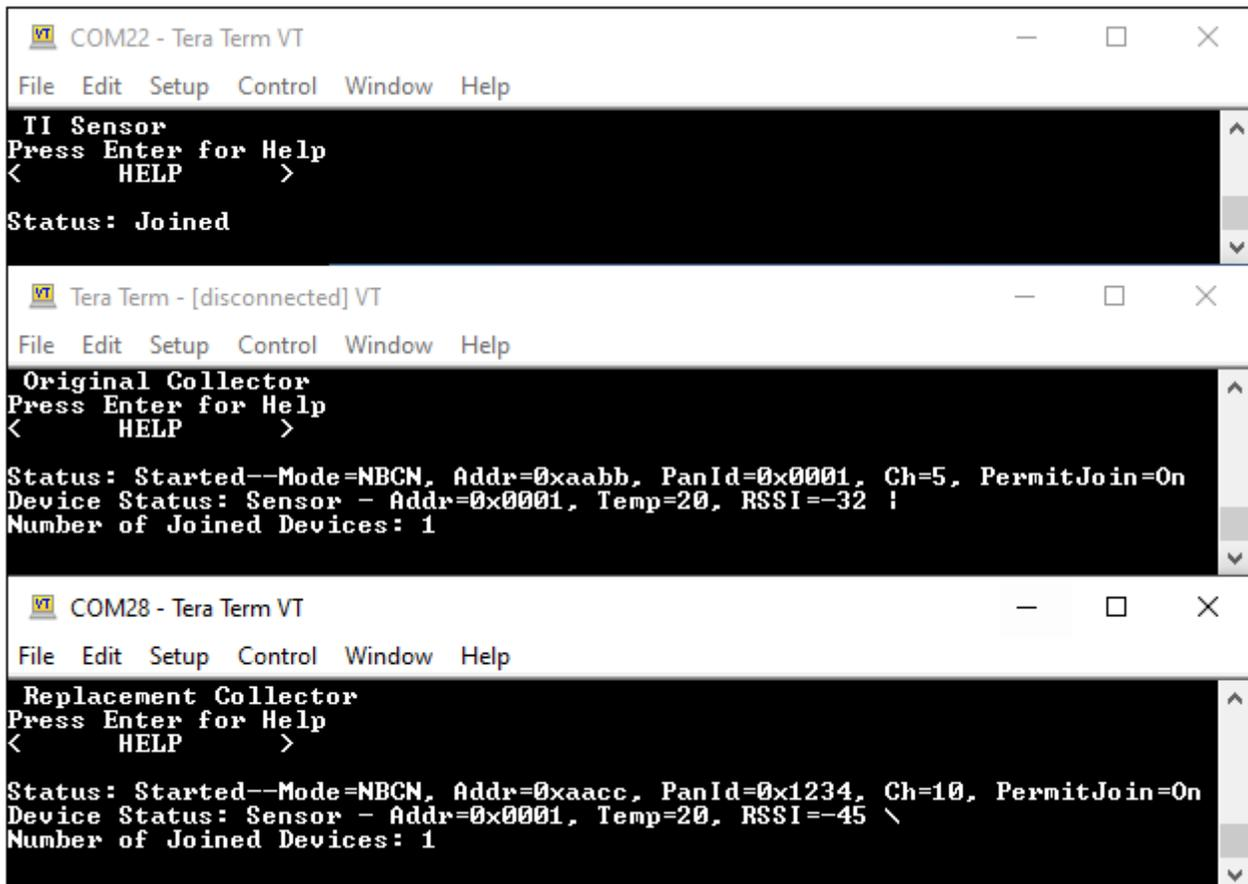
Figure 6-8. Common User Interface for the Sensor and Two Collectors After the First Collector is Disconnected
