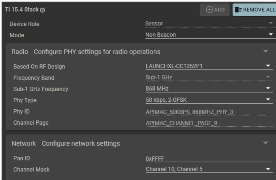
**Figure 6-4. TI 15.4-Stack SysConfig Configuration for Sensor Device**
