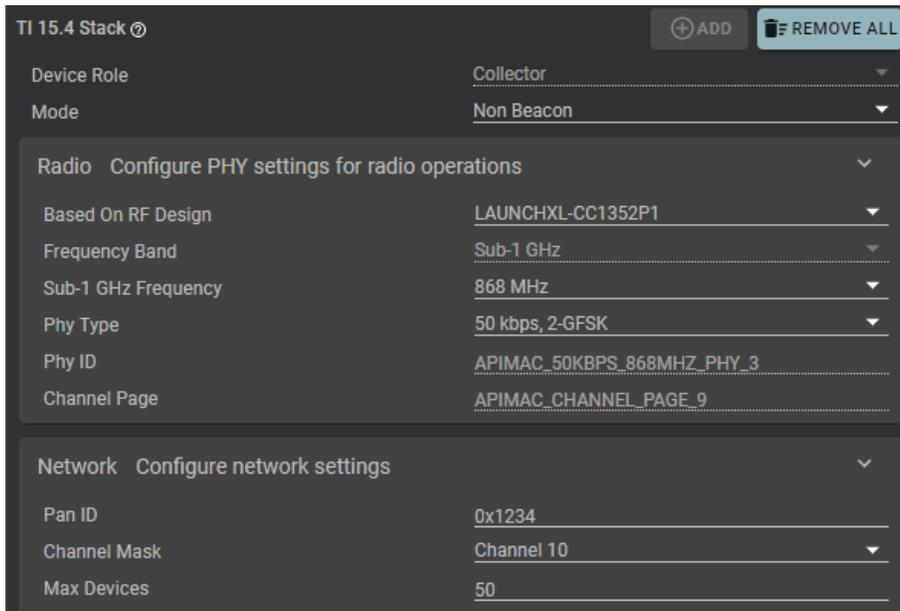
**Figure 6-3. TI 15.4-Stack SysConfig Configuration for Second Collector Device**
