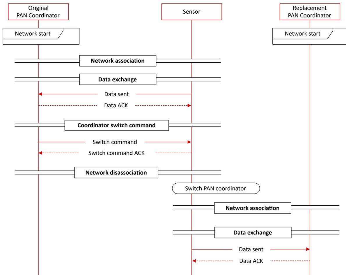
NOTE: This sequence does not cover communication between the local gateways and the central gateway.
