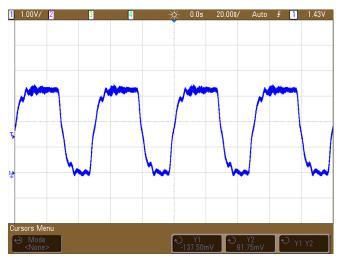
Figure 21. Clock Signal Probed At Modulator 2 - Single Series Termination
