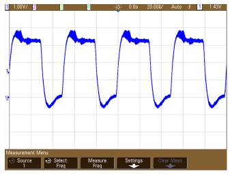
Figure 44. Clock Signal Probed At Modulator 2 -Individual Series Termination
