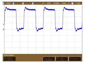
Figure 5. Clock Signal Probed at Buffer Output - No Termination
