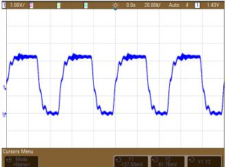
Figure 22. Clock Signal Probed At Modulator 1 - Single Series Termination
