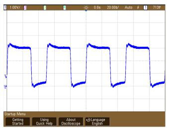
Figure 8. Clock Signal Probed at Buffer Output -Thevenin Termination
