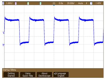
Figure 34. Clock Signal Probed At Buffer Output -Thevenin AC Termination
