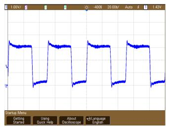
Figure 31. Clock Signal Probed At Buffer Output -Thevenin AC Termination
