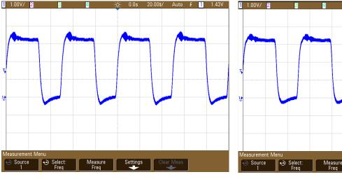
Figure 40. Clock Signal Probed At Modulator 2 -Individual Series Termination
