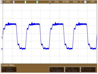
Figure 20. Clock Signal Probed At Modulator 3 - Single Series Termination
