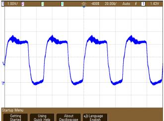
Figure 32. Clock Signal Probed At Modulator 3 -Thevenin AC Termination
