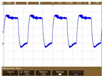
Figure 45. Clock Signal Probed At Modulator 1 -Individual Series Termination
