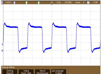
Figure 9. Clock Signal Probed at Modulator 3 - Thevenin Termination
