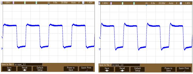
Figure 11. Clock Signal Probed at Buffer Output -Thevenin AC Termination
