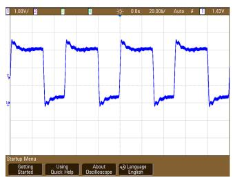
Figure 36. Clock Signal Probed At Buffer Output -Thevenin AC Termination
