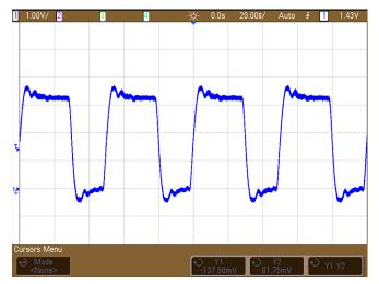
Figure 14. Clock Signal Probed At Buffer Output - No Termination
