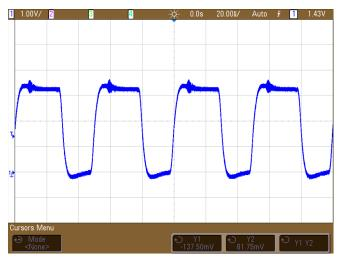
Figure 23. Clock Signal Probed At Buffer Output -Individual Series Termination
