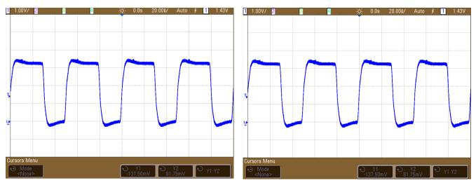
Figure 25. Clock Signal Probed At Modulator 2 -Individual Series Termination
