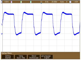
Figure 35. Clock Signal Probed At Modulator 3 -Thevenin AC Termination
