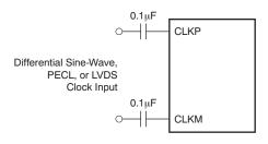
Figure 113. Differential Clock Driving Circuit
