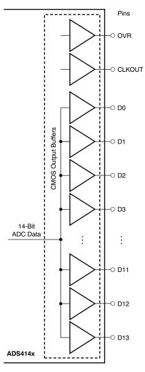
Figure 101. CMOS Output Interface
