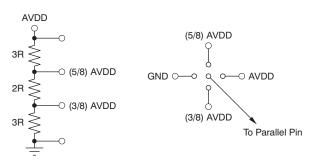
Figure 103. Simplified Diagram to Configure DFS Pin
