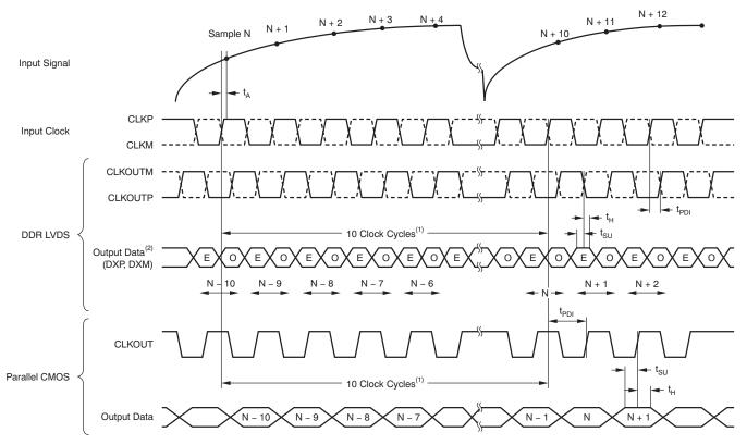
(1) ADC latency in low-latency mode. At higher sampling frequencies,  $t_{DPI}$  is greater than one clock cycle which then makes the overall latency = ADC latency + 1.
