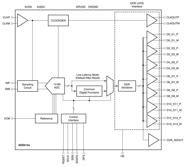
Figure 94. ADS414x Block Diagram
