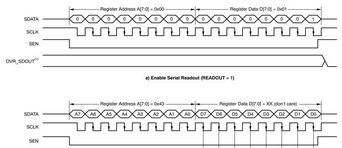
b) Read Contents of Register 0x43. This Register Has Been Initialized with 0x40 (device is put into global power-down mode).
