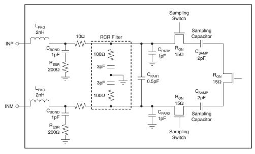
Figure 105. Analog Input Equivalent Circuit
