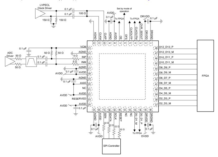
Figure 114. Example Schematic for ADS414x
