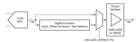
Figure 95. Digital Processing Block Diagram
