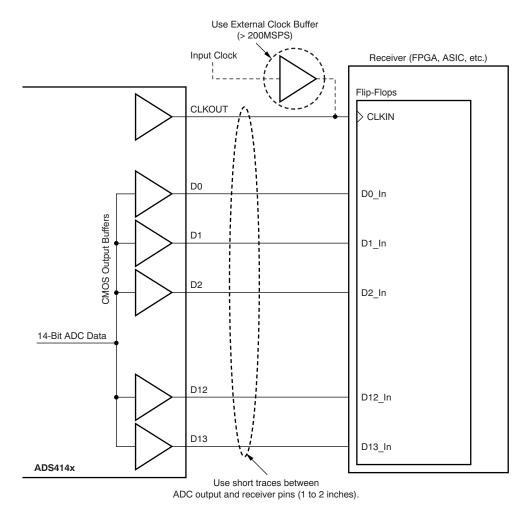
Figure 102. Using the CMOS Data Outputs
