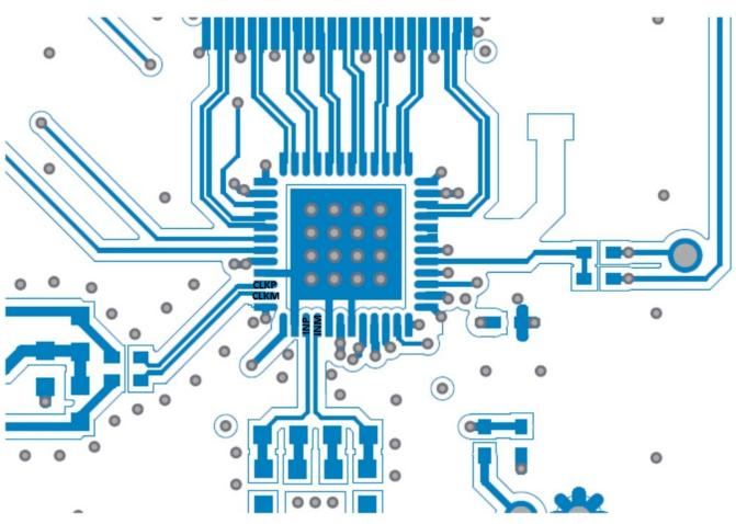
Figure 116. ADS412x and ADS414x EVM PCB Layout
