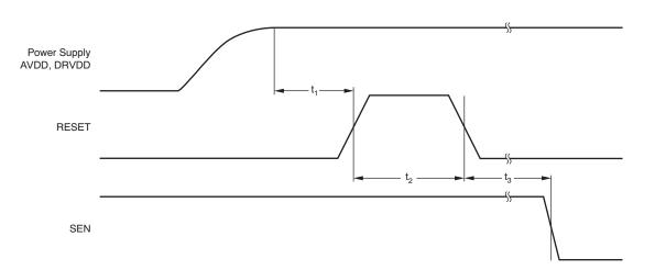
A high pulse on the RESET pin is required in the serial interface mode in case of initialization through hardware reset. For parallel interface operation, RESET must be permanently tied high.
