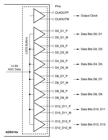
Figure 98. ADS414x LVDS Data Outputs
