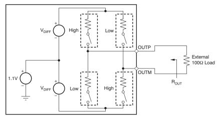
Use the default buffer strength to match 100- $\Omega$  external termination (R<sub>OUT</sub> = 100  $\Omega$ ). To match with a 50- $\Omega$  external termination, set the LVDS STRENGTH bit (R<sub>OUT</sub> = 50  $\Omega$ ).
