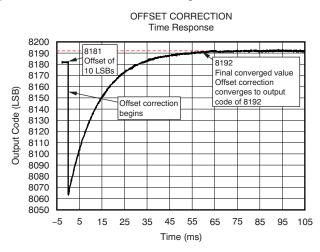
Figure 96. Time Response of Offset Correction
