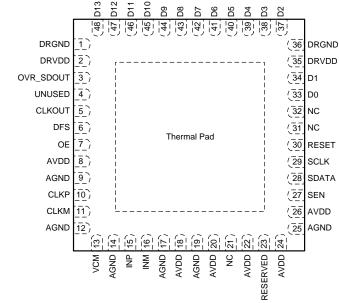
The thermal pad is connected to DRGND.
