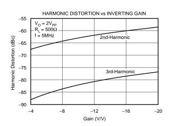
$T_A$  = +25°C, G = +6,  $R_F$  = 750 $\Omega$ , and  $R_L$  = 500 $\Omega$ ,  $V_H$  = - $V_L$  = 2V, unless otherwise noted.
