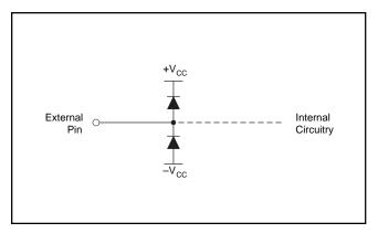
FIGURE 18. I/O Pin ESD Protection.
