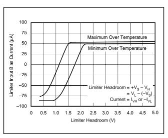
FIGURE 12. Limiter Bias Current vs Bias Voltage.
