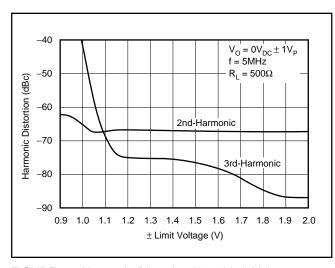
FIGURE 13. Harmonic Distortion Near Limit Voltages.
