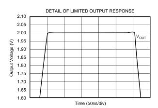
$T_A = +25^{\circ}C$ , G = +6,  $R_F = 750\Omega$ , and  $R_L = 500\Omega$ ,  $V_H = -V_L = 2V$ , unless otherwise noted
