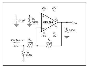
FIGURE 3. Inverting G = -4 Specifications and Test Circuit.
