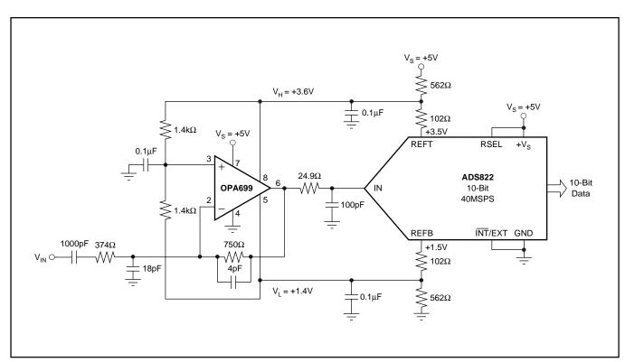
FIGURE 6. Single Supply, Limiting ADC Input Driver.
