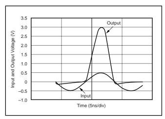
FIGURE 9. 100MHz Sinewave Rectified.
