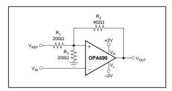
FIGURE 10. Very High-Speed Schmitt Trigger.
