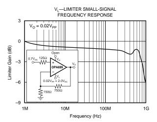
$T_A = +25^{\circ}C$ , G = +6,  $R_F = 750\Omega$ , and  $R_L = 500\Omega$ ,  $V_H = -V_L = 2V$ , unless otherwise noted.
