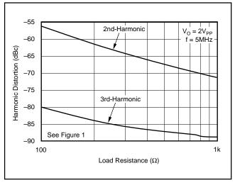
FIGURE 15. 5MHz Harmonic Distortion vs Load Resistance.
