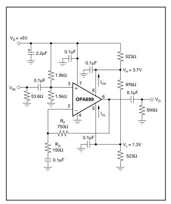
FIGURE 2. AC-Coupled, Single-Supply Amplifier.
