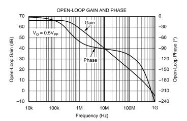
$T_A = +25^{\circ}C$ , G = +6,  $R_F = 750\Omega$ , and  $R_L = 500\Omega$ ,  $V_H = -V_L = 2V$ , unless otherwise noted.
