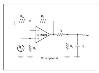
FIGURE 14. Driving Capacitive Loads.
