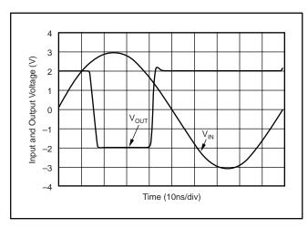
FIGURE 11. Schmitt Trigger Time Domain Response for a 10MHz Sinewave.
