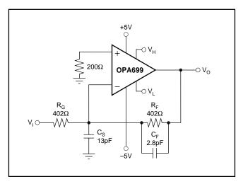
FIGURE 5. Broadband, Low-Inverting Gain External Compensation.
