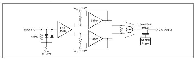
Figure 61. Basic CW Processing Block Diagram
