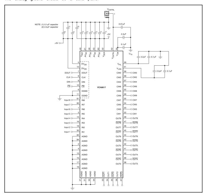
Figure 67. Basic Connection Diagram
