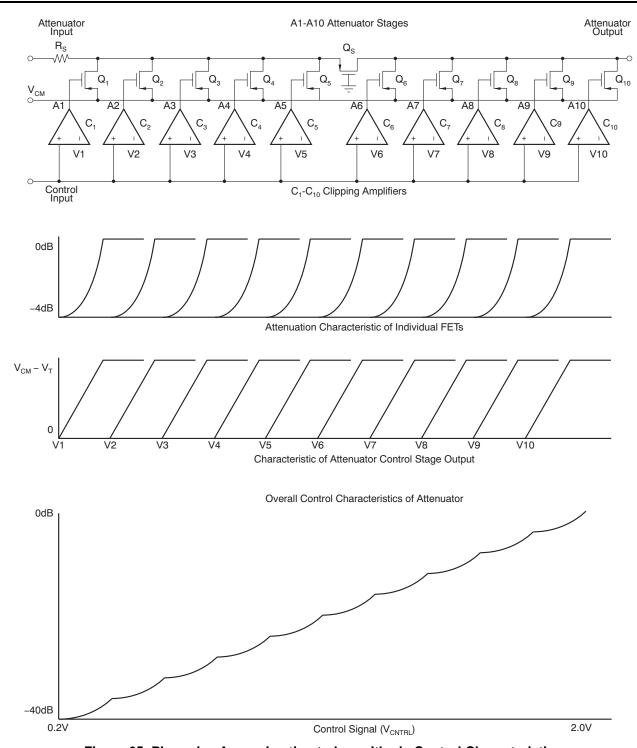
Figure 65. Piecewise Approximation to Logarithmic Control Characteristics
