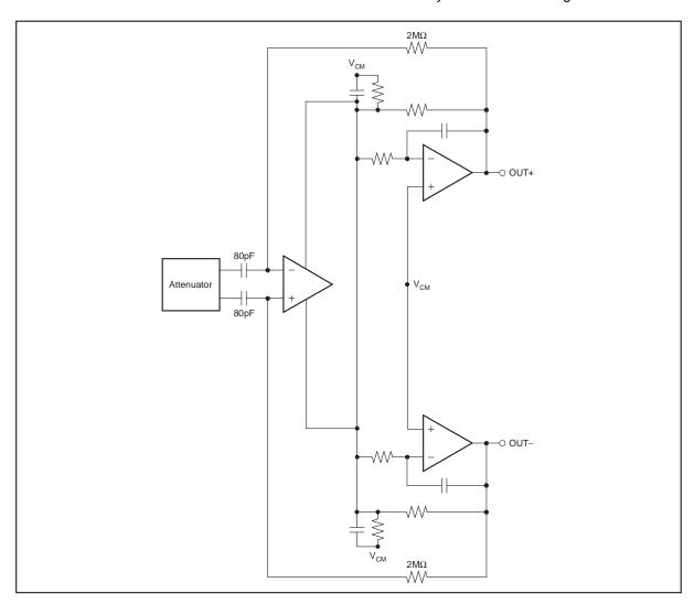
Figure 66. Simplified PGA and Output Filter Circuit
