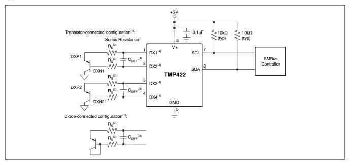
(1) Diode-connected configuration provides better settling time. Transistor-connected configuration provides better series resistance cancellation.
