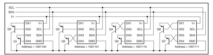
Figure 13. TMP422 Connections for Device Address Setup
