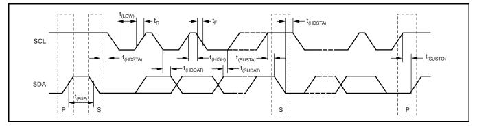
Figure 14. Two-Wire Timing Diagram
