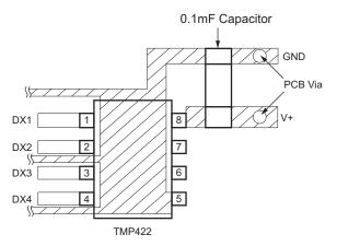
Figure 19. Suggested Bypass Capacitor Placement and Trace Shielding
