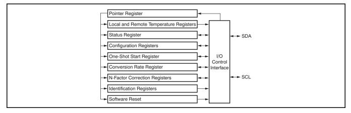
Figure 12. Internal Register Structure
