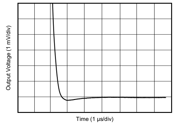
Figure 5-26. Large-Signal Settling Time (Negative)
