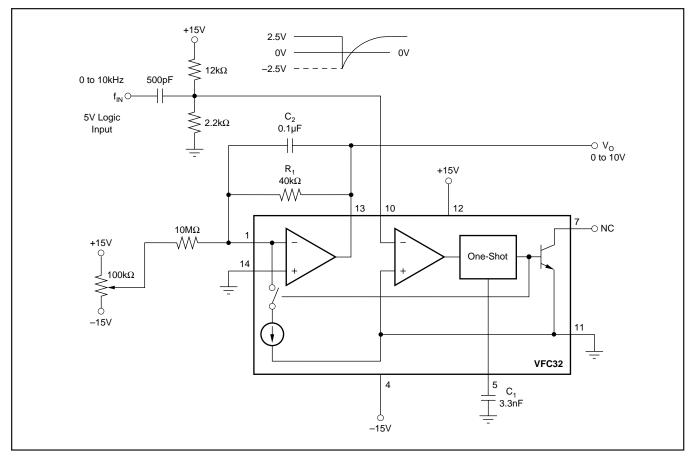
FIGURE 4. Frequency-to-Voltage Converter Circuit.
