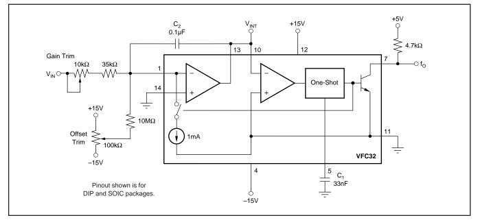
FIGURE 3. Gain and Offset Voltage Trim Circuit.
