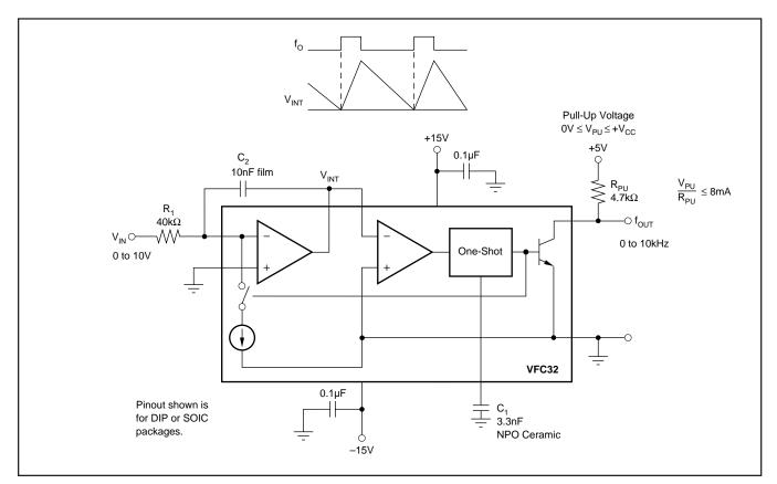
FIGURE 1. Voltage-to-Frequency Converter Circuit.
