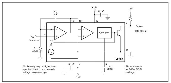
FIGURE 5. V/F Converter—Negative Input Voltage.
