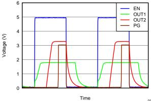
Figure 30. Power Sequence with SEQ = L
