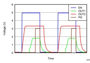
Figure 31. Power Sequence with SEQ = H
