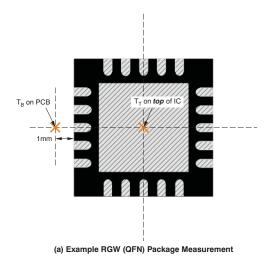
Figure 35. Measuring Points for  $T_T$  and  $T_B$
