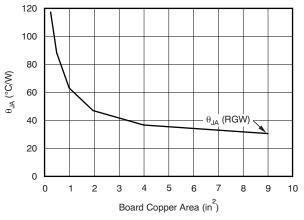
NOTE:  $\theta_{JA}$  value at a board size of 9-in<sup>2</sup> (that is, 3-in × 3-in) is a JEDEC standard.
