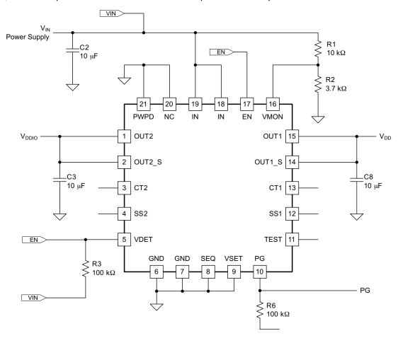
Figure 25. Configuration for F280x, F281x, F223x and F2833x Controllers (Set to automatically sequence C2000 when  $V_{IN} > 4.5 \text{ V}$ ) (C2, C3, C8 / 10- $\mu$ F X5R ceramic capacitors)
