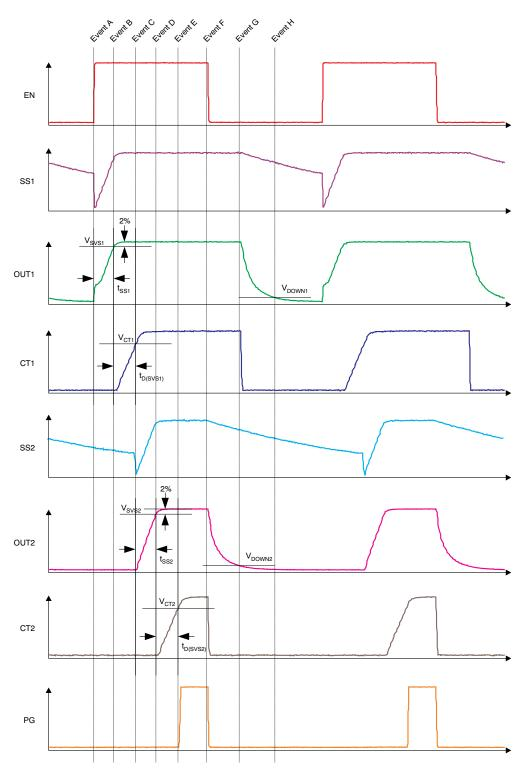
Figure 32. Normal Power-Up and Power-Down Timing
