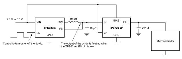
Figure 25. Floating IN Pin Regulation Example
