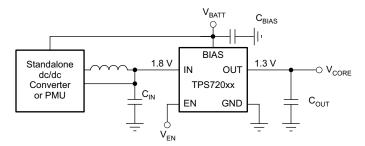
Figure 26. Typical Application Schematic
