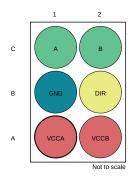
Figure 4-4. YZP Package, 6-Pin DSBGA (Bottom View)
