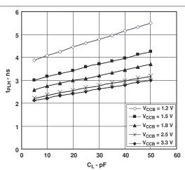
Figure 5-2. Typical Propagation Delay of Low-to-High (A to B) vs Load Capacitance  $T_A = 25^{\circ}C$ ,  $V_{CCA} = 1.2V$
