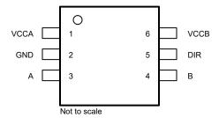
Figure 4-3. DRL Package, 6-Pin SOT-5X3 (Top View)
