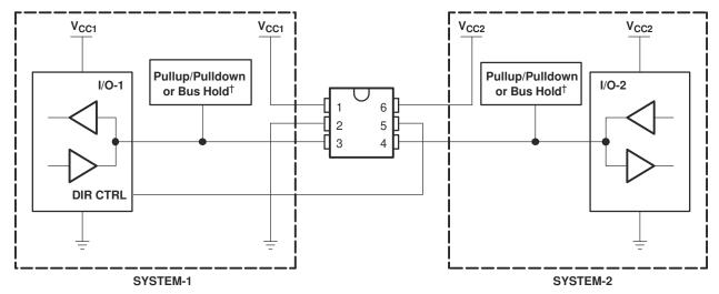
Figure 8-3. Bidirectional Logic Level-Shifting Application
