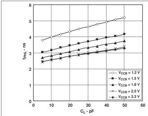
Figure 5-1. Typical Propagation Delay of High-to-Low (A to B) vs Load Capacitance  $T_A = 25^{\circ}C$ ,  $V_{CCA} = 1.2V$
