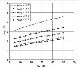
Figure 5-10. Typical Propagation Delay of Low-to-High (A to B) vs Load Capacitance  $T_A = 25^{\circ}\text{C}, \, V_{CCA} = 3.3\text{V}$
