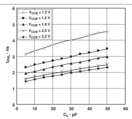
Figure 5-8. Typical Propagation Delay of Low-to-High (A to B) vs Load Capacitance  $T_A = 25^{\circ}C$ ,  $V_{CCA} = 2.5V$
