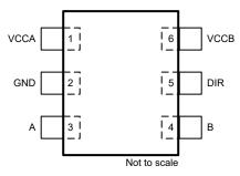
Figure 4-2. DCK Package, 6-Pin SOT-SC70 (Top View)
