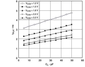
Figure 5-7. Typical Propagation Delay of High-to-Low (A to B) vs Load Capacitance  $T_A = 25^{\circ}C$ ,  $V_{CCA} = 2.5V$
