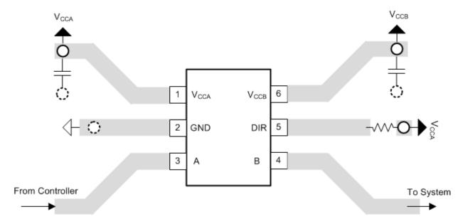
Figure 8-5. PCB Layout Example
