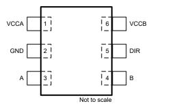
Figure 4-1. DBV Package, 6-Pin SOT-23 (Top View)
