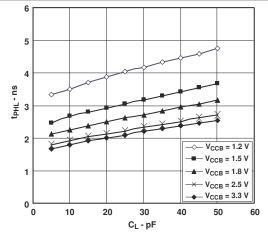
Figure 5-6. Typical Propagation Delay of Low-to-High (A to B) vs Load Capacitance  $T_A = 25^{\circ}C$ ,  $V_{CCA} = 1.8V$
