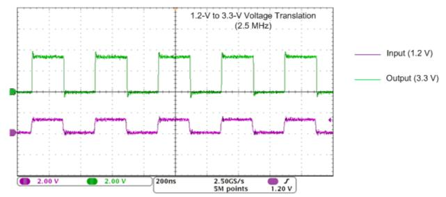
Figure 8-4. Translation Up (1.2V to 3.3V) at 2.5MHz
