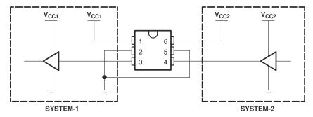
Figure 8-1. Unidirectional Logic Level-Shifting Application
