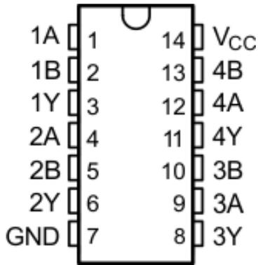
Figure 4-1. D, DB, DGV, N, NS, PW, or W Package 14-Pin SOIC, SSOP, TVSOP, PDIP, SO, or TSSOP (Top View)
