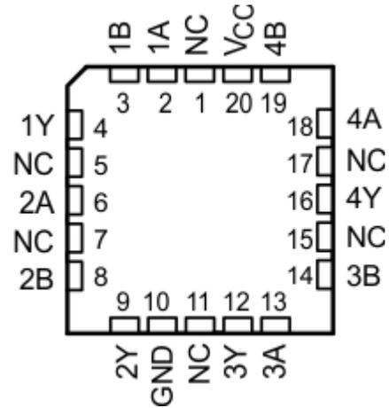
Figure 4-2. FK Package 20-Pin LCCC (Top View)
