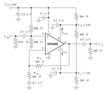
Figure 31. AC-Coupled, Single Supply Amplifier
