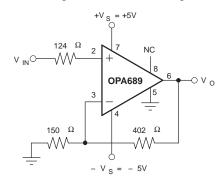
Figure 33. Precision Half Wave Rectifier
