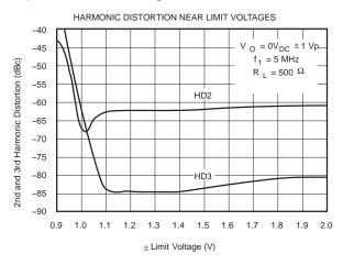
Figure 37. Harmonic Distortion Near Limit Voltages
