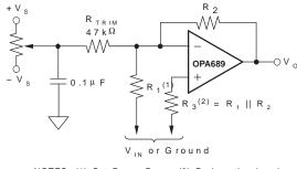
NOTES: (1) Set  $R_1 << R_{TRIM}$ . (2)  $R_3$  is optional and minimizes output offset due to input bias currents.
