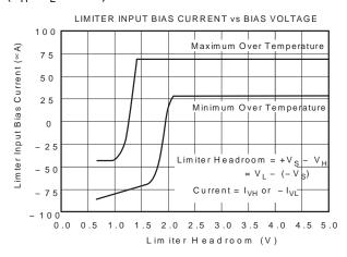
Figure 36. Limiter Bias Current vs Bias Voltage
