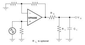
Figure 39. Driving Capacitive Loads
