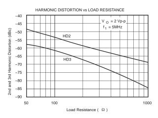
Figure 40. 5-MHz Harmonic Distortion vs Load Resistance
