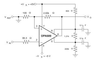
Figure 34. Very High Speed Comparator
