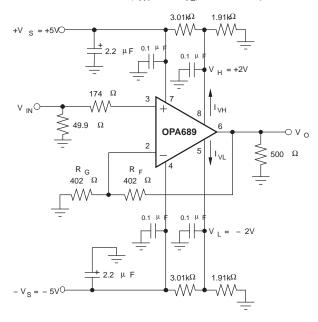
Figure 30. DC-Coupled, Dual Supply Amplifier
