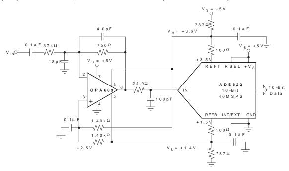
Figure 32. Low Distortion, Limiting ADC Input Driver
