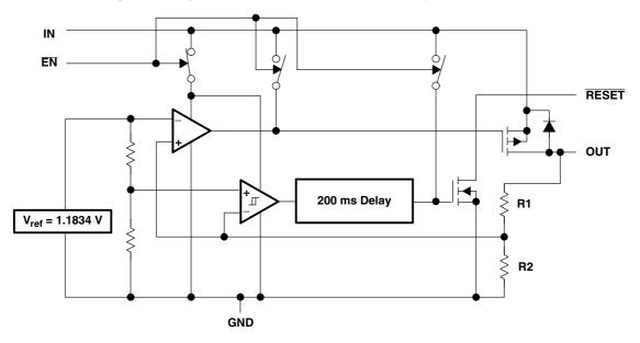
functional block diagram—fixed-voltage version (for each LDO)
