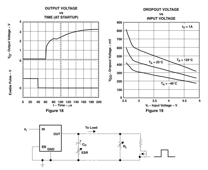
Figure 20. Test Circuit for Typical Regions of Stability (Figures 21 through 24) (fixed output options)
