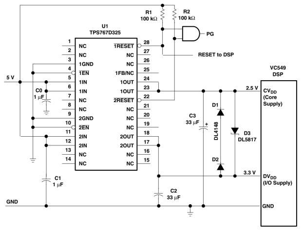
Figure 25. Dual-Voltage DSP Application
