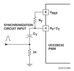
Figure 2. Oscillator Synchronization Circuit
