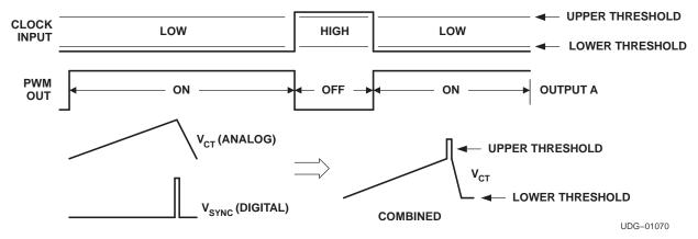
Figure 3. Synchronization to an External Clock
