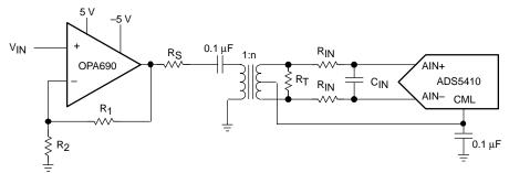
Figure 23. Converting a Single-Ended Input Signal Into a Differential Signal Using an RF Transformer
