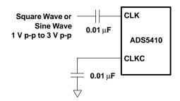
Figure 26. AC-Coupled Single-Ended Clock Input
