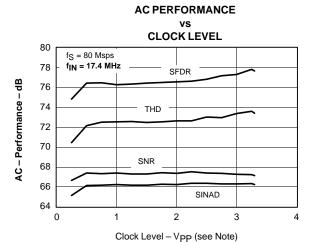
NOTE: Voltage peak to peak in pin 19 or 20. Multiply by 2 to obtain differential peak to peak.
