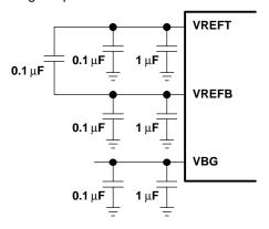
Figure 25. Internal Reference Usage
