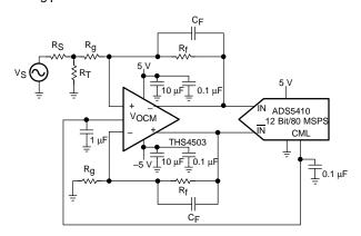
Figure 24. Using the THS4503 With the ADS5410
