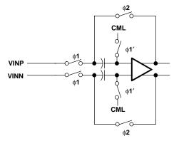
Figure 19. Analog Input Stage
