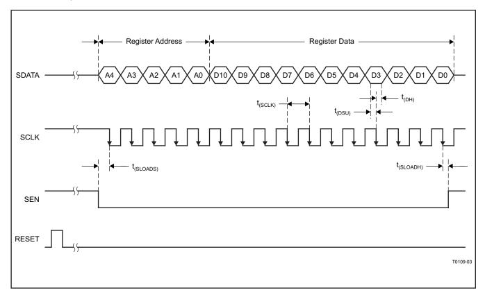
Figure 4. Serial Interface Timing
