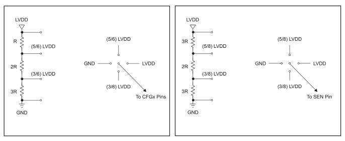
Figure 3. Simple Scheme to Configure Parallel Pins
