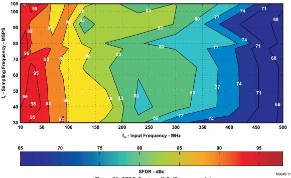
Figure 76. SFDR Contour (3.5 dB coarse gain)
