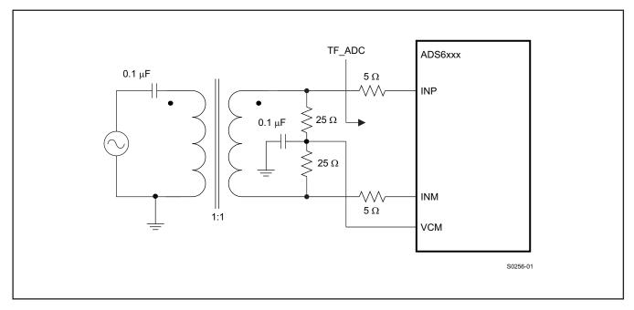
Figure 82. Single Transformer Drive Circuit
