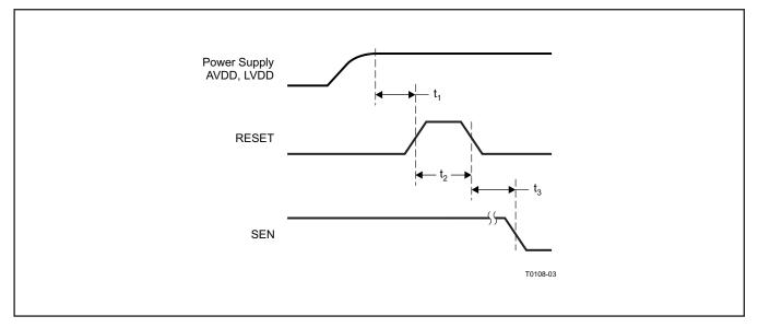
Figure 5. Reset Timing
