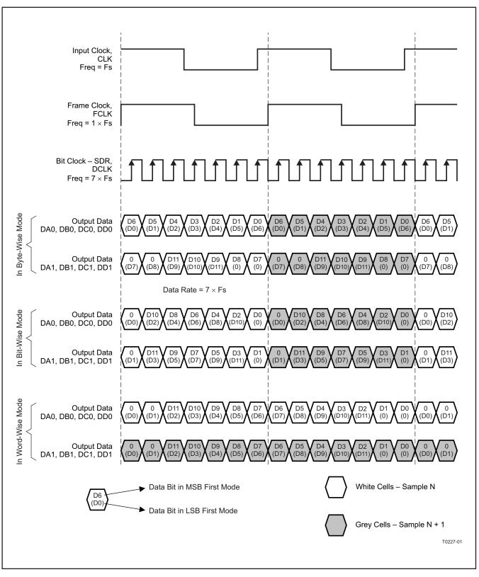
Figure 93. 2-Wire Interface 14× Serialization – SDR Bit Clock
