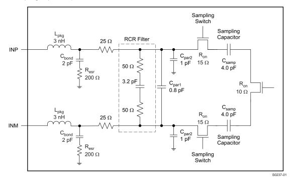
Figure 79. Input Sampling Circuit
