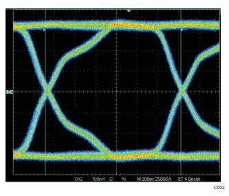
Figure 96. LVDS Data Eye Diagram with 10-pF Load Capacitance (100 Ω Internal Termination)
