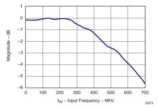
Figure 80. Analog Input Bandwidth
