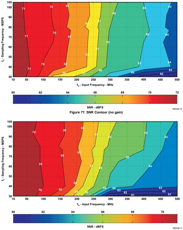
Figure 78. SNR Contour (3.5 dB coarse gain)
