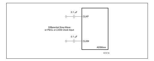
Figure 88. Differential Clock Driving Circuit
