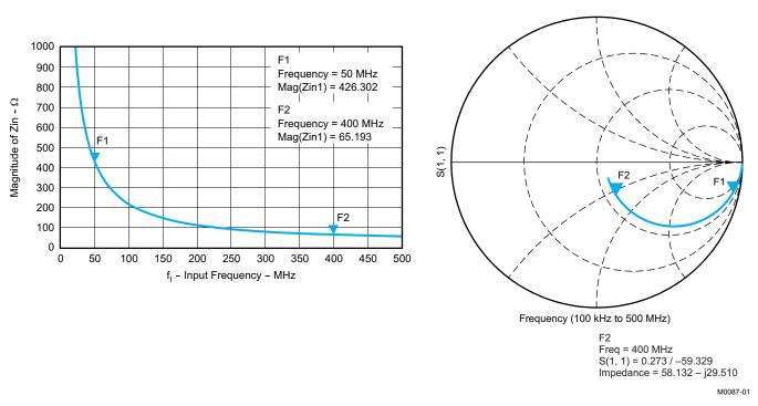
Figure 81. ADC Input Impedance, Zin
