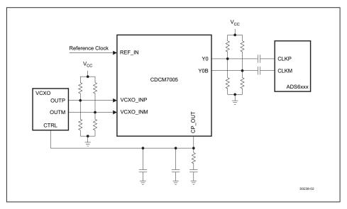
Figure 89. PECL Clock Drive Using CDCM7005
