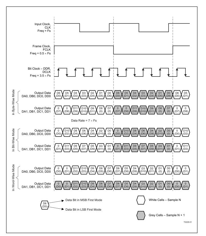
A. In the byte-wise and bit-wise modes, the frame clock frequency is 1 x Fs. In the word-wise mode, the frame clock frequency is 0.5 x Fs
