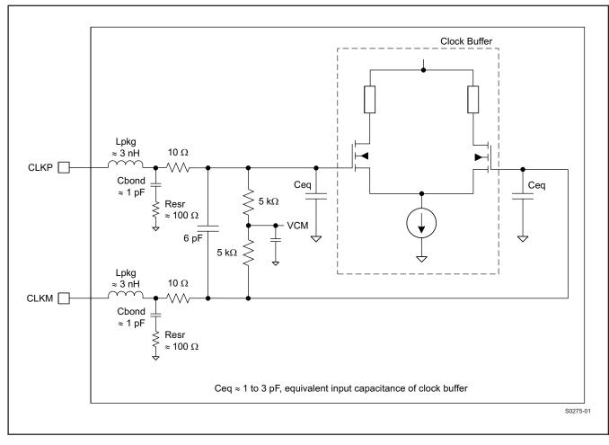
Figure 86. Internal Clock Buffer
