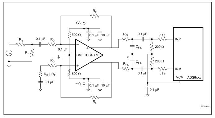
Figure 84. Drive Circuit using THS4509
