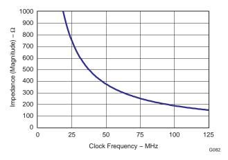
Figure 87. Clock Buffer Input Impedance
