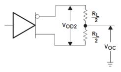
Figure 6-1. Driver V<sub>OD2</sub> and V<sub>OC</sub>
