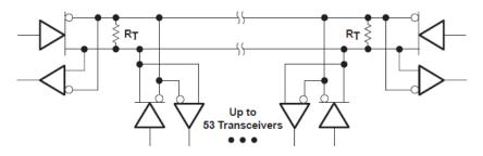
A. The line should terminate at both ends in its characteristic impedance (R<sub>T</sub> = Z<sub>0</sub>). Stub lengths off the main line should be kept as short as possible.
