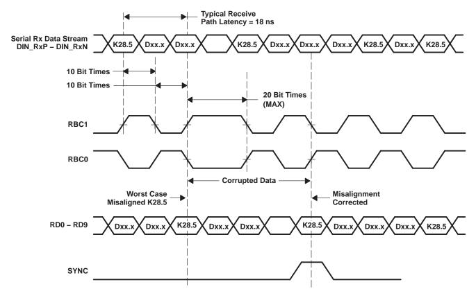
Figure 2. Word Realignment Timing Characteristics Waveforms
