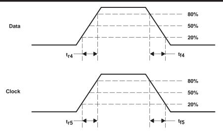
Figure 6. Receiver Data Measurement Levels
