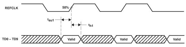
Figure 4. Transmit 10-Bit Interface Timing Waveforms
