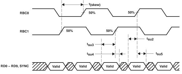
Figure 7. Receiver Interface Timing Waveforms
