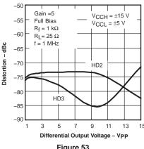
**DIFFERENTIAL DISTORTION** vs **DIFFERENTIAL OUTPUT VOLTAGE**
