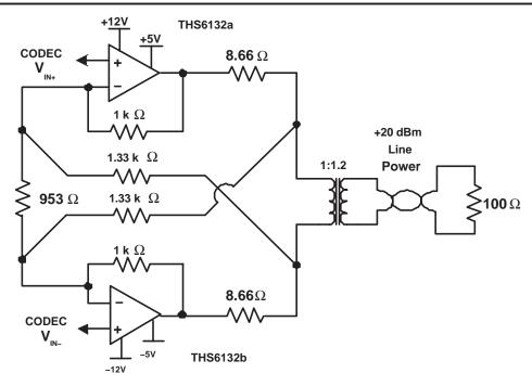
Figure 1. ±12 V Active Termination ADSL CO Line Driver Circuit (Synthesis Factor = 4; CF = 5.6)
