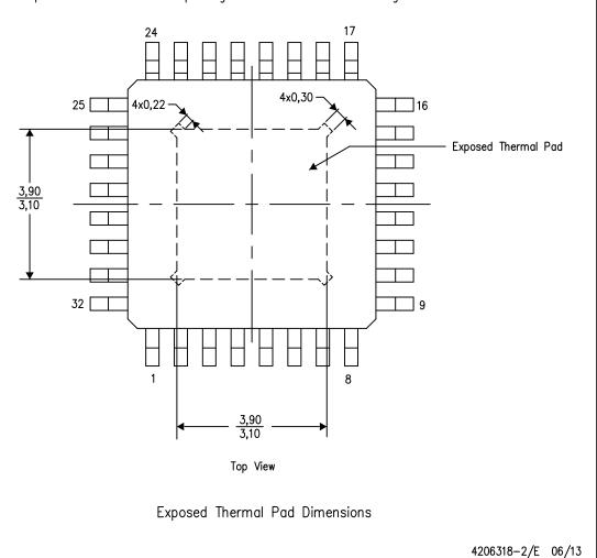
NOTE: All linear dimensions are in millimeters
