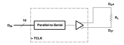
$V_{OD} = (D_0+) - (D_0-)$ Differential Output Signal Is Shown as  $(D_0+) - (D_0-)$
