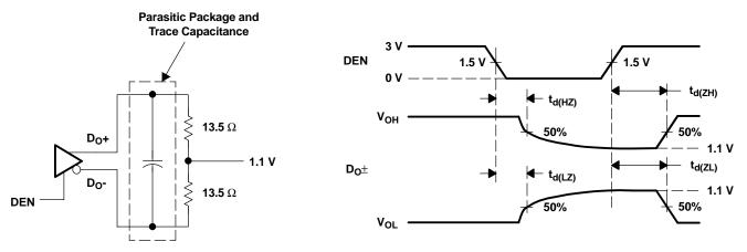
Figure 9. Serializer High-Impedance-State Test Circuit and Timing
