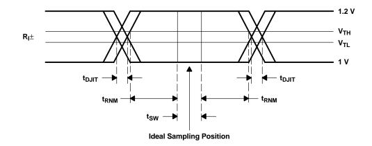
$t_{SW}$ : Setup and Hold Time (Internal Data Sampling Window)  $t_{DJIT}$ : Serializer Output Bit Position Jitter That Results From Jitter on TCLK  $t_{RNM}$ : Receiver Noise Margin Time
