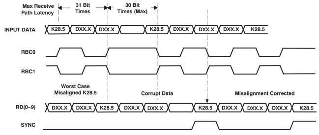
Figure 5. Word Realignment Timing Characteristics Waveforms
