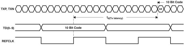
Figure 1. Transmitter Latency Full Rate Mode
