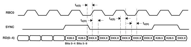
Figure 4. Synchronous Timing Characteristics Waveforms (DDR mode)
