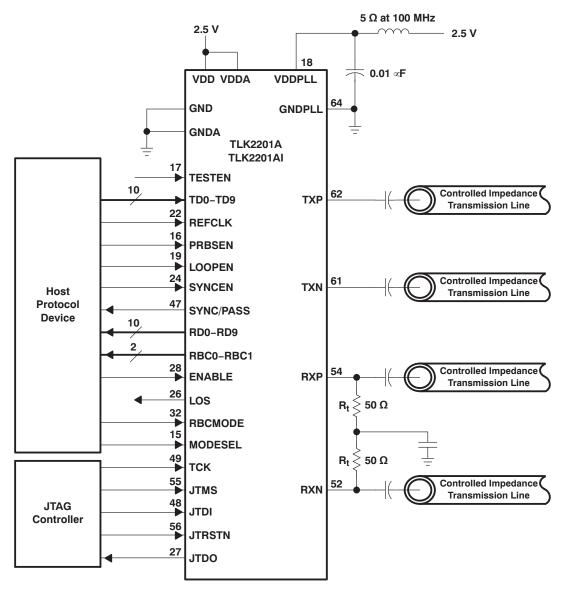
Figure 12. Typical Application Circuit (AC mode)
