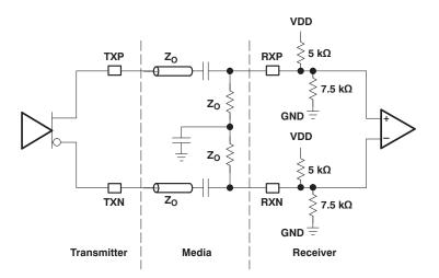
Figure 11. High-Speed I/O AC-Coupled Mode
