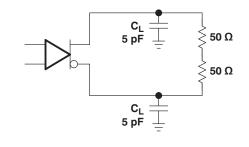
Figure 8. Transmitter Test Setup
