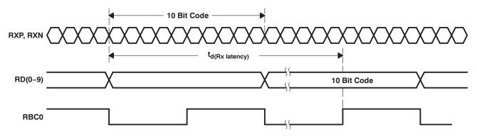
Figure 6. Receiver Latency – TBI Normal Mode Shown
