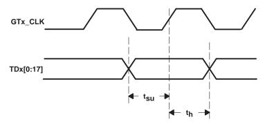
Figure 1. Transmit Timing Waveform
