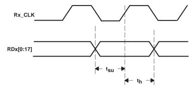
Figure 4. Receive Timing Waveform
