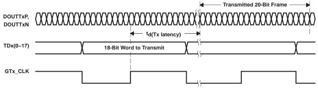
Figure 2. Transmitter Latency
