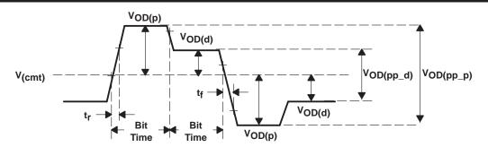
Figure 8. Differential and Common-Mode Output Voltage Definitions
