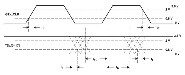
Figure 6. TTL Data Input Valid Levels for AC Measurements
