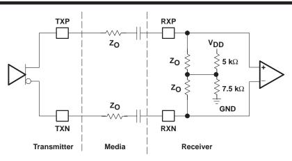
Figure 11. High-Speed I/O AC-Coupled Mode
