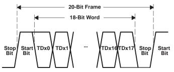
Figure 3. Serial Output Data Stream With Start and Stop Bit
