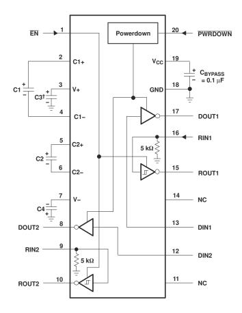
$<sup>^\</sup>dagger$  C3 can be connected to  $V_{\mbox{\footnotesize CC}}$  or GND.
