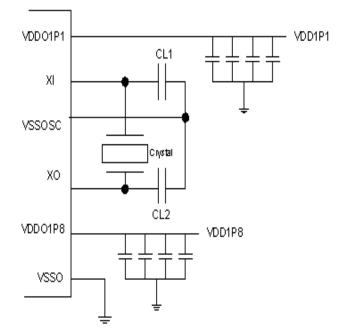
Figure 5-1. Typical Crystal Connections
