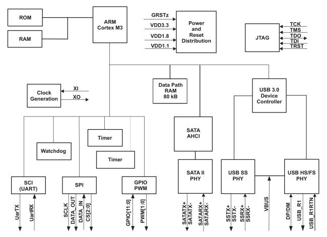
Figure 2-1. Device Block Diagram
