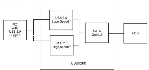
(1) USB connection is made at either SuperSpeed or High-Speed depending on the upstream connection support.
