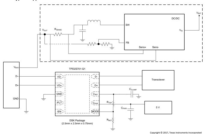
Figure 21. USB 2.0 Port With Short-to-V<sub>BUS</sub> and IEC ESD Protection
