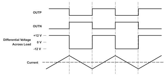
Figure 20. Traditional Class-D Modulation Scheme's Output Voltage and Current Waveforms into an Inductive Load With No Input
