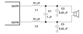
Figure 23. Typical LC Output Filter, Cutoff Frequency of 27 kHz, Speaker Impedance = 4  $\Omega$
