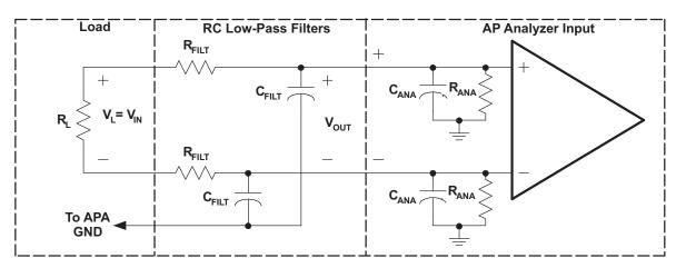
Figure 30. Measurement Low-Pass Filter Derivation Circuit-Class-D APAs
