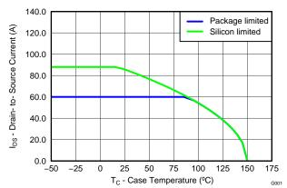
Figure 13. Maximum Drain Current vs. Temperature
