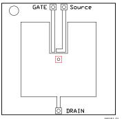
Max  $R_{\theta JA} = 50^{\circ}C/W$ when mounted on 1 inch2 (6.45 cm2) of 2oz. (0.071-mm thick) Cu.
