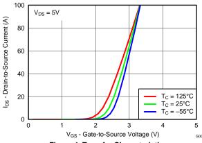
Figure 4. Transfer Characteristics
