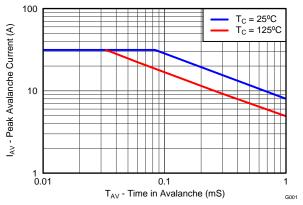
Figure 12. Single Pulse Unclamped Inductive Switching
