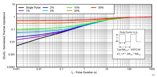
Figure 2. Transient Thermal Impedance
