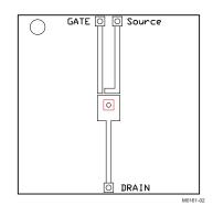
Max  $R_{\theta JA} = 125^{\circ}C/W$ when mounted on a minimum pad area of 2-oz. (0.071-mm thick) Cu.
