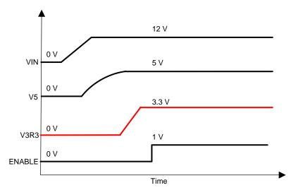
Figure 123. Power Supply Waveforms
