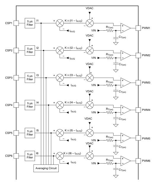
Figure 15. AutoBalance Current Sharing Circuit Detail
