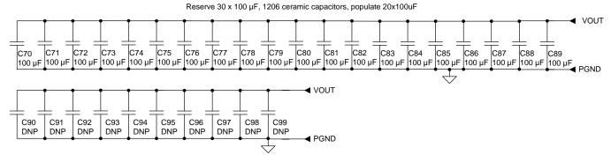
Figure 105. Input and Output Filter for a 6-Phase, 1 V, 180 A Application
