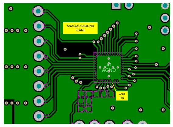
Figure 128. Layout Example for TPS53667 Grounding
