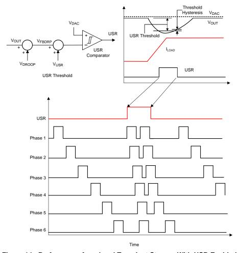
Figure 14. Performance for a Load Transient Step-up With USR Enabled
