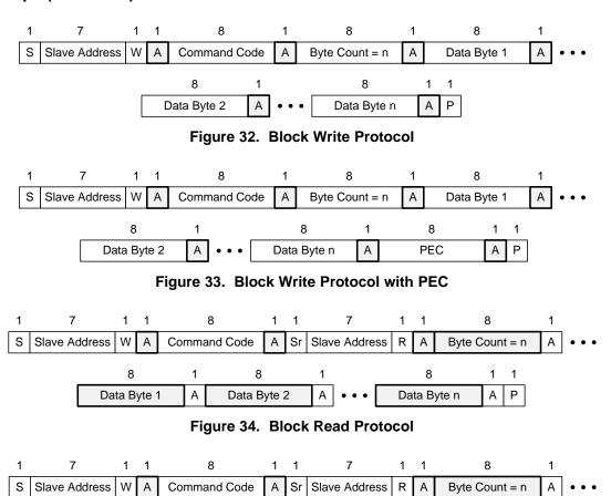
Figure 35. Block Read Protocol with PEC
