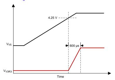
Figure 7. V3R3 Startup Waveform
