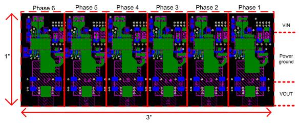
Figure 129. Layout Example of Power Density
