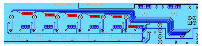
Figure 126. Layout Example for PWM Traces
