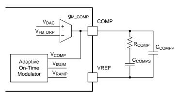
Figure 106. Compensation Circuitry
