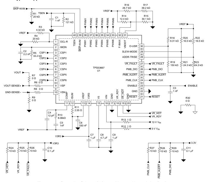
Figure 103. Controller Schematic for a 6-Phase, 1 V, 180 A Application
