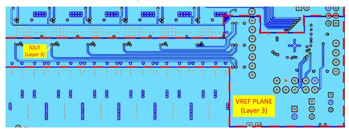
Figure 124. Layout Example of Current Sensing Traces
