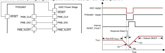
Figure 17. RESET Pin Connection
