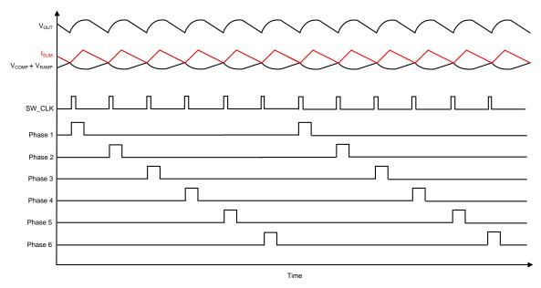
Figure 8. D-CAP+ Mode Basic Waveforms
