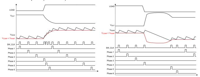
Figure 10. Load Insertion
