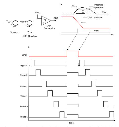
Figure 13. Performance for a Load Transient Release with OSR Enabled
