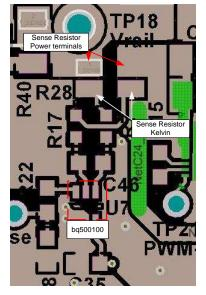
Figure 20. Current Sensing Layout
