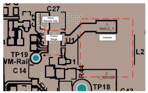
Figure 17. V\_RAIL Power Stage Layout
