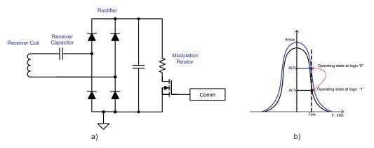
Figure 7. Receiver Resistive Modulation Circuit
