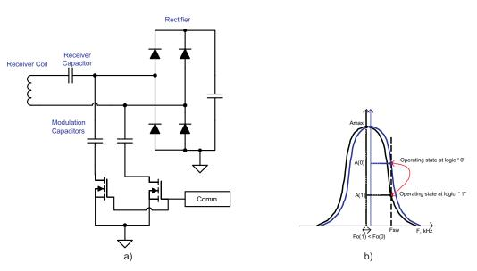
Figure 8. Receiver Capacitive Modulation Circuit
