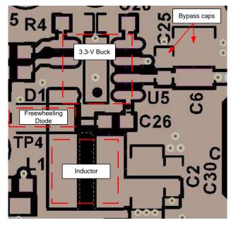
Figure 14. 3.3-V DC-DC Buck Regulator Layout
