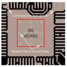
Figure 16. Continuous GND Layout
