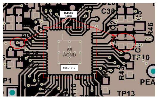
Figure 15. Bypass Capacitors Layout
