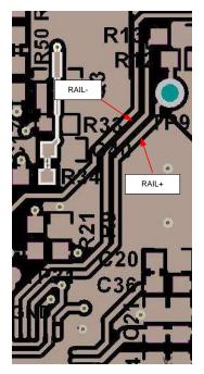
Figure 21. Balanced Differential Signal Layout
