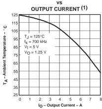
(1) Safe operating area is applicable to the test board conditions listed in the dissipation rating table section of this data sheet.
