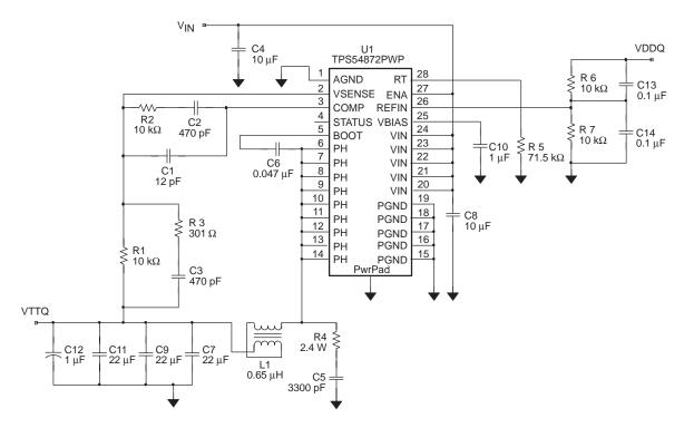
Figure 7. Application Circuit
