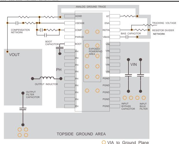
Figure 8. TPS54872 PCB Layout
