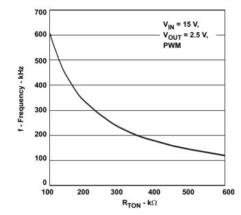
Figure 19. Switching Frequency vs R<sub>TON</sub>
