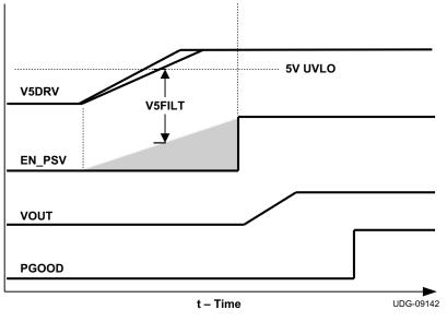
Figure 20. Start-Up Timing Sequence
