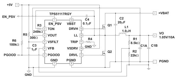
Figure 25. 1.05-V/10-A Application from VBAT (RGY Package)
