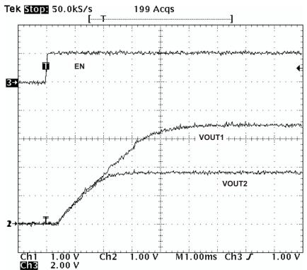
Figure 39. Simultaneous Startup With Tracking Resistor
