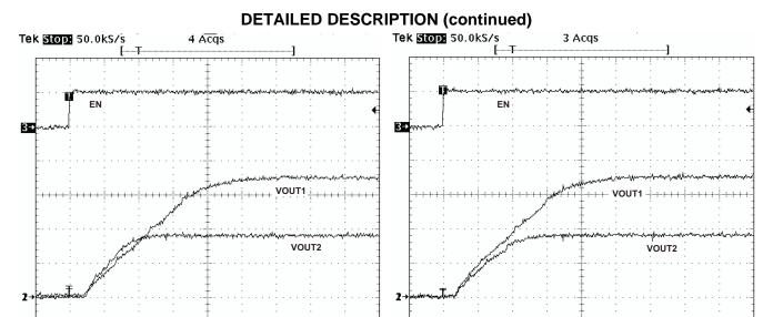
Figure 37. Ratiometric Startup with VOUT2 leading Figure 38. Ratiometric Startup with VOUT1 leading VOUT2
