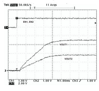
Figure 35. Ratio-Metric Startup using Coupled SS/TR pins
