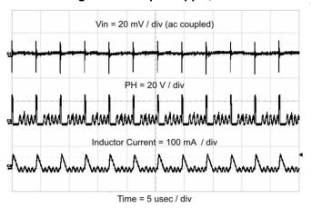
Figure 57. Input Ripple CCM
