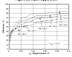
Figure 59. Efficiency vs Load Current
