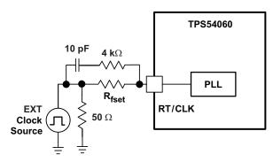
Figure 43. Synchronizing to a System Clock
