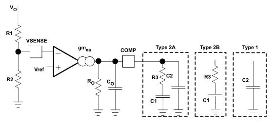
Figure 49. Types of Frequency Compensation
