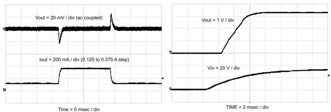
Figure 52. Load Transient
