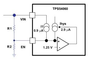
Figure 28. Adjustable Undervoltage Lockout (UVLO)
