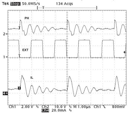
Figure 46. Plot of Synchronizing in PSM
