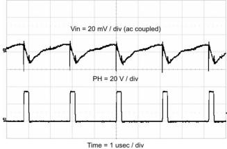
Figure 56. Output Ripple, PSM
