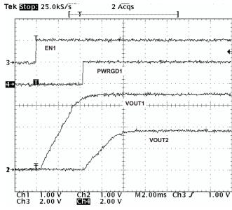
Figure 32. Schematic for Sequential Start-Up Sequence
