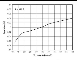
Figure 63. Regulation vs Input Voltage
