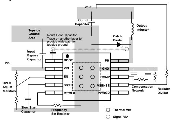
Figure 64. PCB Layout Example
