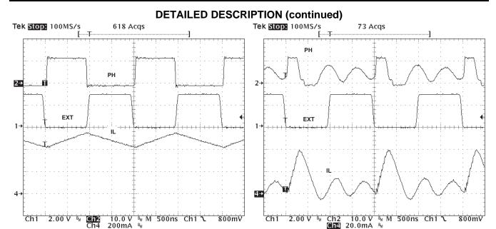
Figure 44. Plot of Synchronizing in ccm
