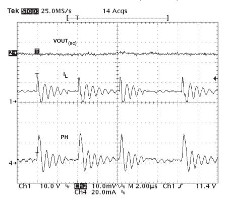
Figure 25. Pulse Skip Mode Operation
