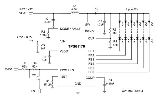
Figure 21. Typical Applications (to Support Separate 1.8-V Logic PWM and EN Signals)
