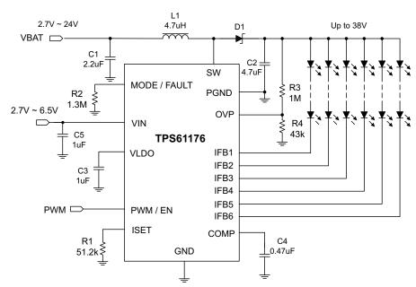
Figure 18. Typical Applications (Multi-Cell Battery Input Application)
