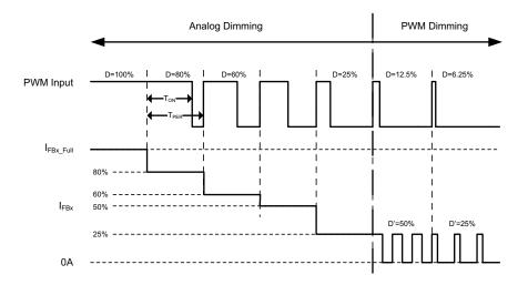
(a). Mixed Dimming Mode with switch point = 25%
