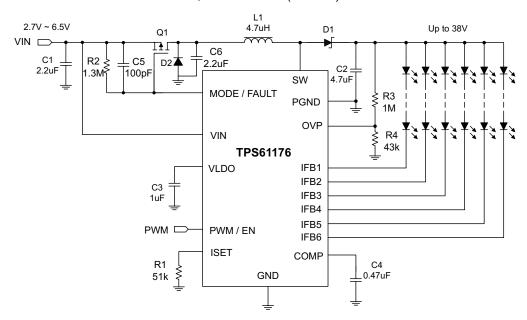
Figure 9. Typical Applications (Single-Cell Battery Input Application)
