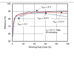
Figure 2. Efficiency vs Dimming Duty Cycle
