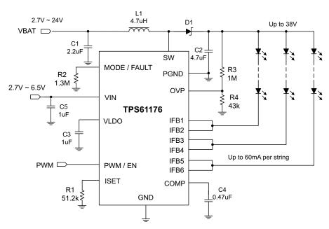
Figure 19. Typical Applications (Combined String to Support High Brightness WLED Diodes)
