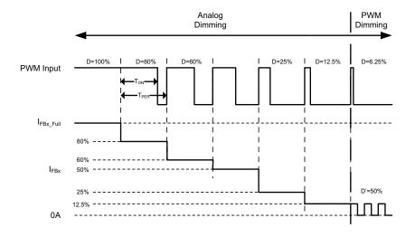
(b). Mixed Dimming Mode with switch point = 12.5%
