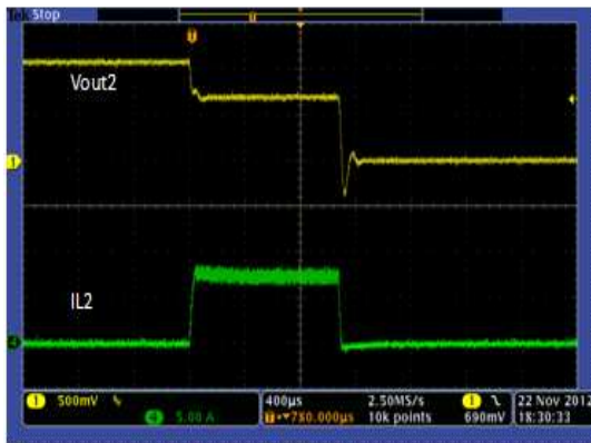
Figure 29. Over Current Protection, Buck 2
