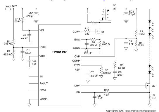
Figure 22. TPS61197 High Boost Ratio Application
