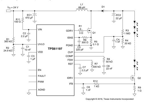
Figure 18. TPS61197 Simple Boost-Converter Application
