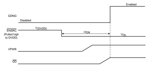
Figure 6. Timing Illustration for  $t_{\rm ON}$
