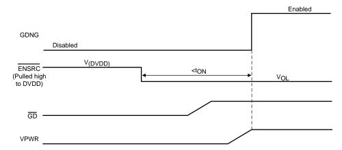
Figure 5. Timing Illustration for ton
