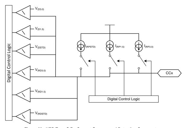
Figure 23. USB Type-C Rp Current Sources and Detection Comparators
