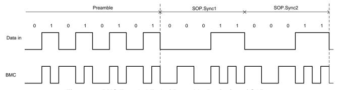
Figure 24. BMC Encoded End of Preamble, Beginning of SOP
