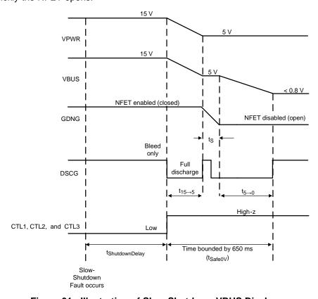
Figure 31. Illustration of Slow-Shutdown VBUS Discharge
