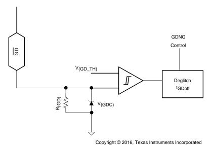
Figure 36. Overcurrent Protection Circuit, (GD)
