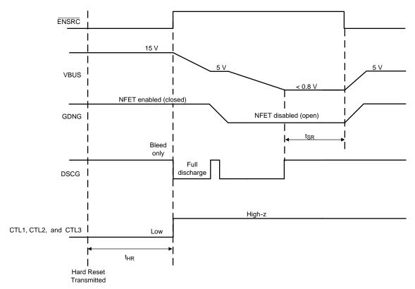
Figure 8. Timing Diagram for ENSRC and GDNG After Transmitting a Hard Reset
