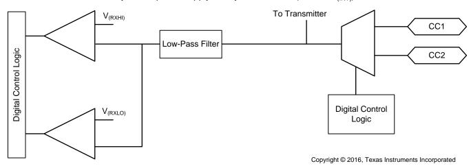
Figure 29. USB PD BMC Receiver Schematic
