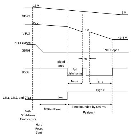
Figure 32. Illustration of Fast-Shutdown Discharge
