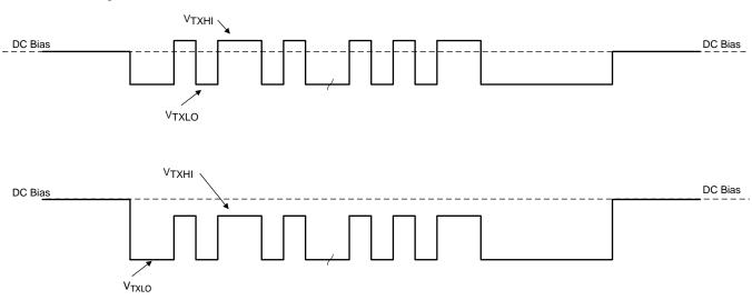
Figure 25. USB PD BMC Transmission on the CC Line
