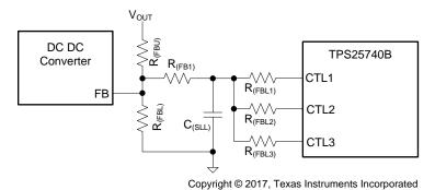
Figure 46. Slew-Rate Control Example No. 3
