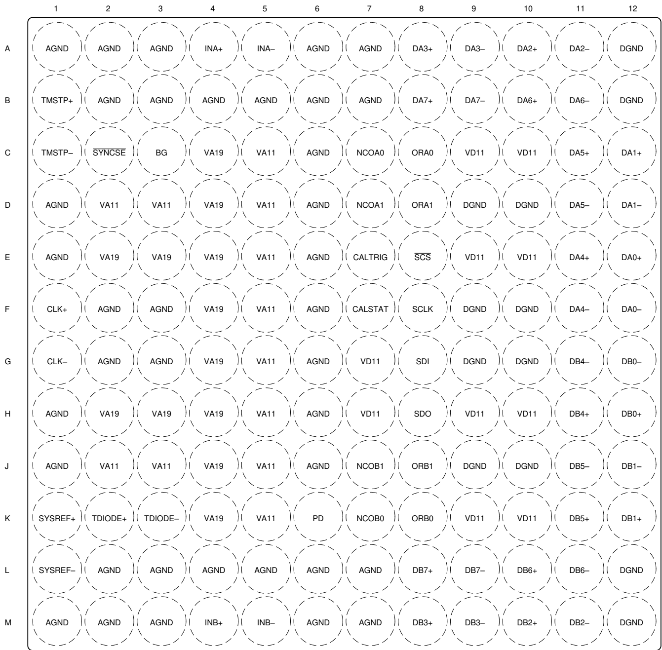
Figure 4-1. AAV Package, 144-Ball Flip Chip BGA Top View
