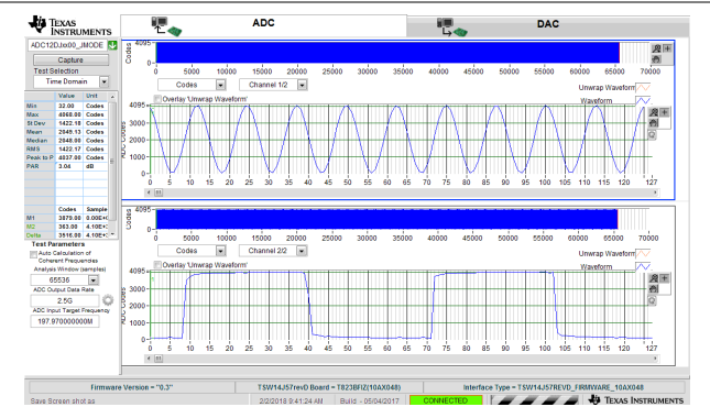
Figure 7-11. 200-MHz, Sine-Wave (Channel A) and 40-MHz, Square-Wave (Channel B) Time Domain for 5-GSPS, Single-Channel Oscilloscope
