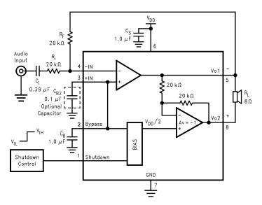
Figure 1. Typical Audio Amplifier Application Circuit
