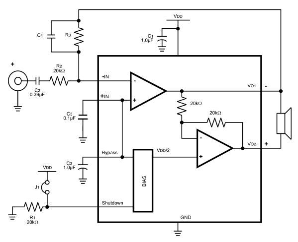
Figure 24. HIGHER GAIN AUDIO AMPLIFIER
