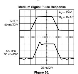
Medium Signal Pulse Response with Capacitive Load
