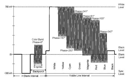
Figure 50. Input Video Signal Before DC Restore Clamp
