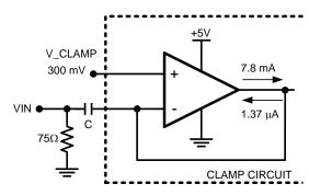
Figure 52. Clamp Circuit
