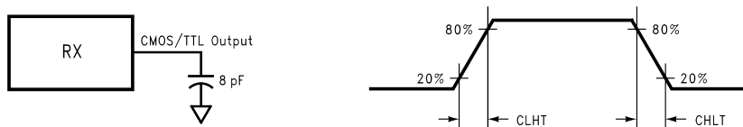
Figure 7. LVC MOS/LVTTL Output Load and Transition Times
