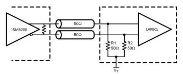
Figure 10. DC Coupled LVDS to LVPECL Interface
