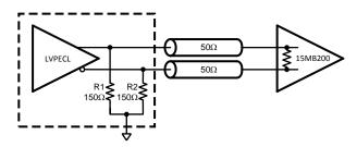
Figure 8. DC Coupled LVPECL to LVDS Interface
