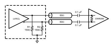
Figure 9. AC Coupled LVPECL to LVDS Interface
