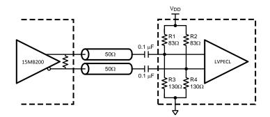
Figure 11. AC Coupled LVDS to LVPECL Interface
