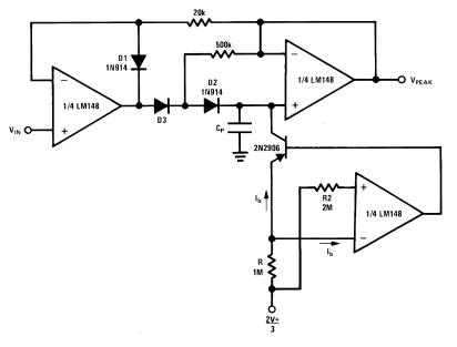
Adjust R for minimum drift D3 low leakage diode D1 added to improve speed  $V_S = \pm 15V$
