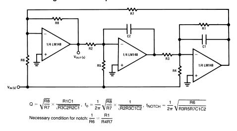
$Ex: f_{NOTCH} = 3 \ kHz, \ Q = 5, \ R1 = 270k, \ R2 = R3 = 20k, \ R4 = 27k, \ R5 = 20k, \ R6 = R8 = 10k, \ R7 = 100k, \ C1 = C2 = 0.001 \ \mu F$
