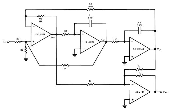
Tune Q through R0, For predictable results:  $f_O Q \le 4 \times 10^4$ Use Band Pass output to tune for Q
