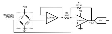
Figure 33. Pressure Sensor Application
