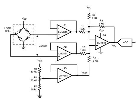
Figure 34. Load Cell Application
