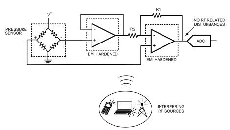
Figure 1. EMI Hardened Sensor Application
