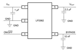
ON/ $\overline{\text{OFF}}$  input must be actively terminated. Tie to V<sub>IN</sub> if this function is not to be used. Minimum output capacitance is shown to insure stability over full load current range. More capacitance provides better dynamic performance and additional stability margin (see Section 7.1.1).
