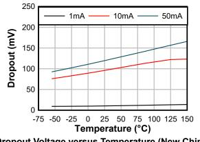
Dropout Voltage versus Temperature (New Chip)
